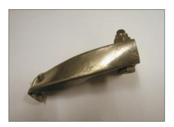
d) The sheet of the end of the wire deflecting cable was deformed towards the left, in the same manner as the deformation noted on the leading edge of the fin. The sheet twisted to the left and broke from its fitting to the fin, which is also coherent with the previous deformations.
