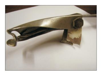
e) The interference of the electric wire with the fin and the significant increase of the curvature of the catenary of the wire deflecting cable show that the rear end of that cable moved due to either the breakage of its fitting to the fin or the breakage of one fitting of the fin base.
