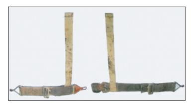
In this regard, it must be taken into account that in addition to atmospheric agents, seat harnesses are also exposed to the chemical substances present in the treatment products used which could modify their properties without significantly altering their appearance.
