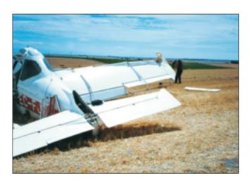
The pilot was fumigating on an irregularly-shaped beet field. A power line ran along the side of the field. Beyond the power line, the land rose forming a hill, with a second power line behind it. The pilot was carrying out the spray runs so that at the end of each run he would pass under the first power line, then immediately climb to clear both the hill and the second power line, and finally turn to begin another spray run.
