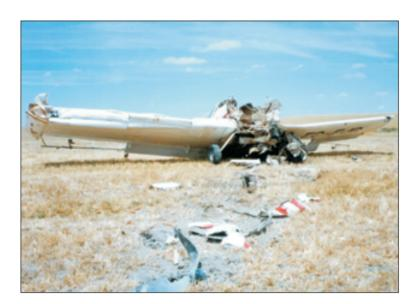
Although no marks of the landing of the aircraft previous to the final impact into the ground were found, due to the fact the area had been subject to intense traffic of vehicles and personnel of the emergency services, that also prepared firebreaks, it is probable that the landing was carried out in a gentle manner, as stated by the pilot.
