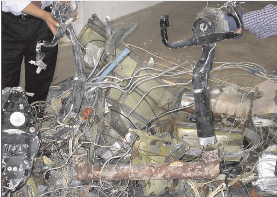
Figure C-4. Control column and rod wreckage
