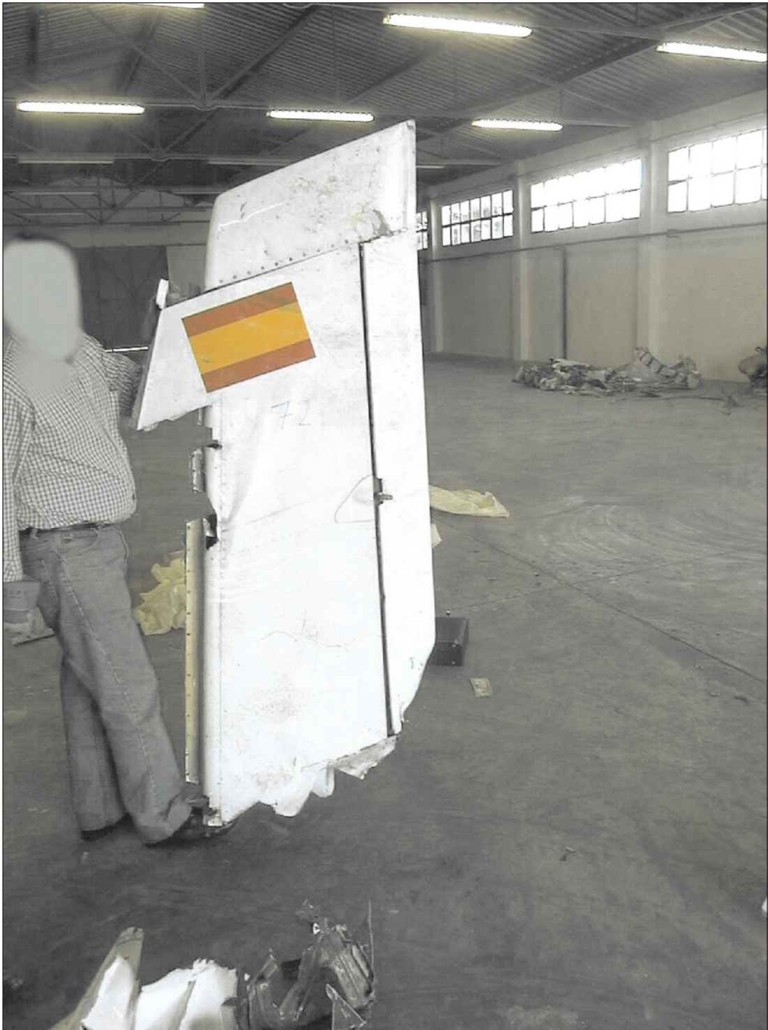
Figure C-1. Vertical fin tail wreckage
