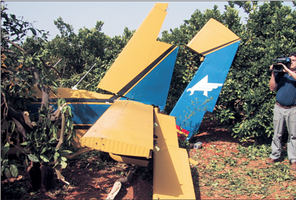
Photo 3. Rudder and elevator broken off
