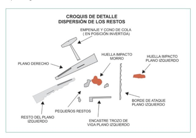
An impact mark was found on the ground, produced by the leading edge of the left wing, and to its left, the impact mark of the aircraft nose was noticed.
