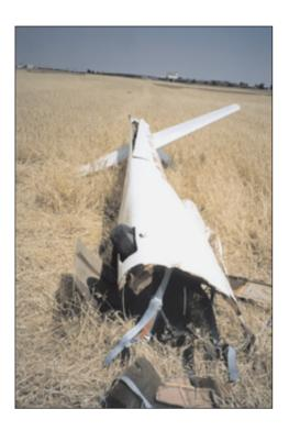
At approximately 17:43, local time, a Robin DR-400-180R aircraft, registration EC-BTN, began to tow a Schleicher Ka 6 BR glider, registration PH-1204, on runway 11 of the Ocaña aerodrome. The take off was carried out in a normal way, the glider lifted off first followed by the towing aircraft shortly afterwards. Seconds later, when both aircraft had travelled about three fourths of the 1200 metrelong runway (see diagram), the tow cable broke.
