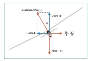
cosine of the angle formed with the vertical  $(\phi)$ , that is to say  $L \cdot \cos \phi$ . Since this value is smaller than L, in order to keep the aircraft from descending, the lift should be increased by increasing the angle of attack. This causes an increase in the induced drag and in the stall speed, i.e. that an aircraft stalls at a higher speed if it is turning than if it were in a straight and level flight.
