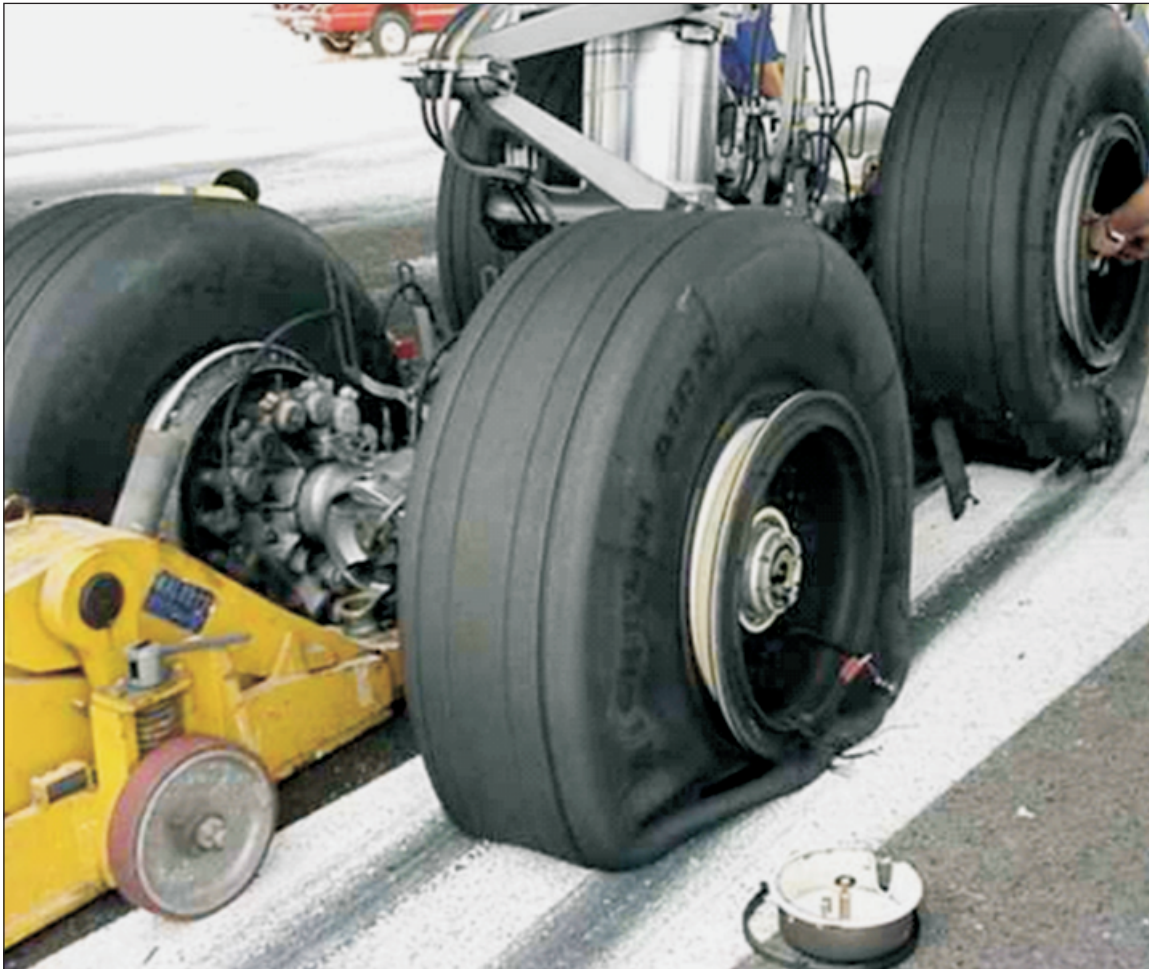
Figure 6. Wheels 3, 4, 7 y 8 (right leg; seen from the rear right angle) after the aircraft stopped on the runway. The white line is the runway side stripe marking of 33. Note the two narrow tracks of every wheel after they burst
