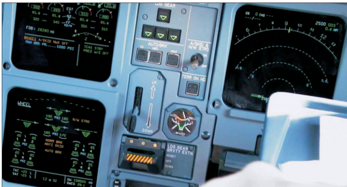
Figure 1. View of the triple indicator of pressure. The landing gear is down, but the antiskid switch is in OFF. Therefore, the vertical bars that represent the brakes of every wheel do not appear in the WHEEL page of the ECAM screen
