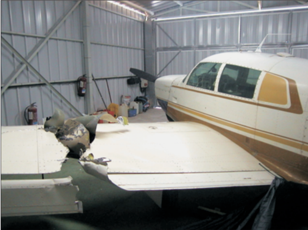
Photography 1. Damages to the left wing. Aircraft D-EIGB
