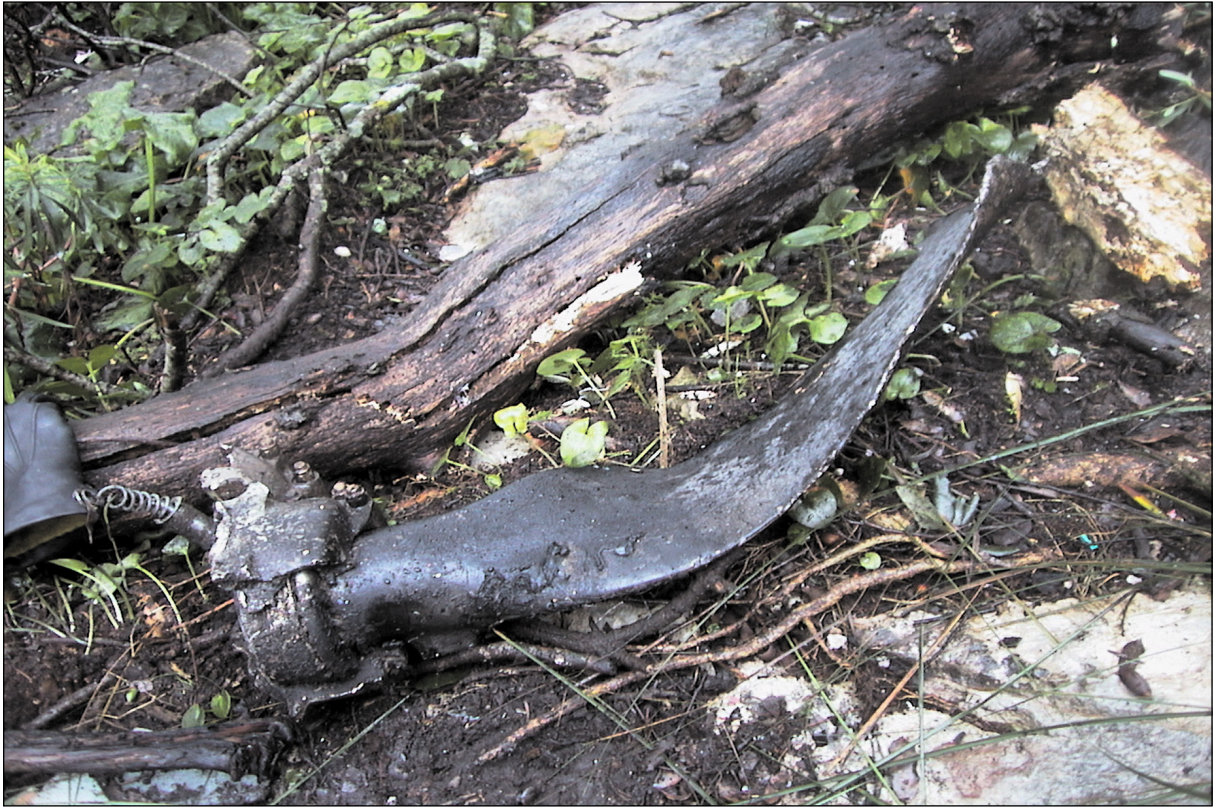
Figure A-3. Wreckage of a propeller blade
