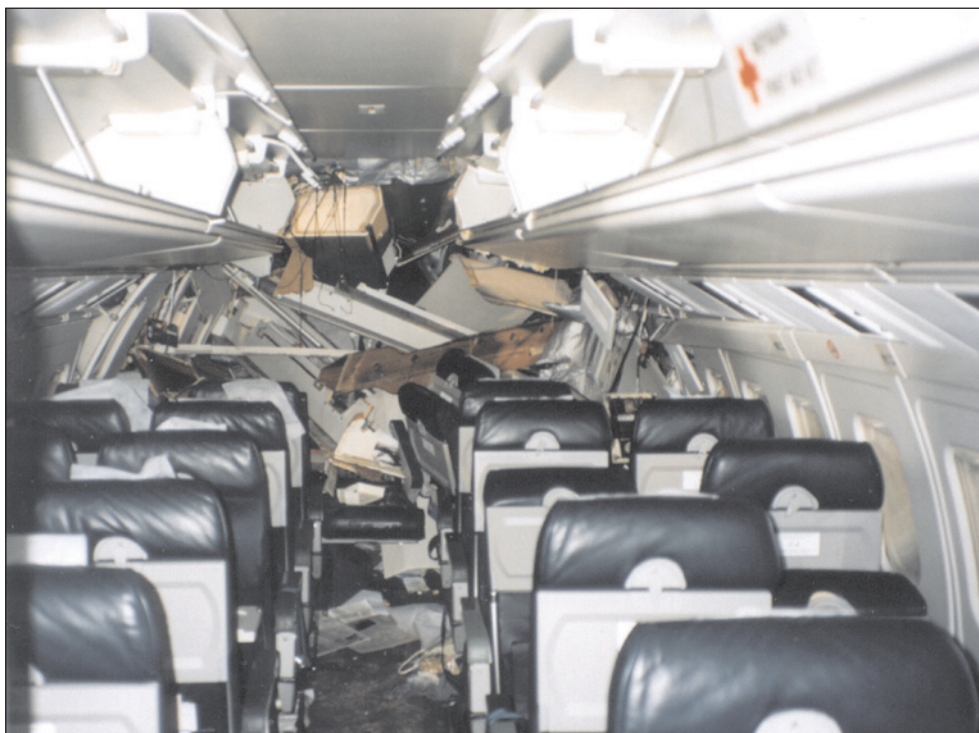
Figure 1.15.2. View of the damage from the rear part of the cabin
