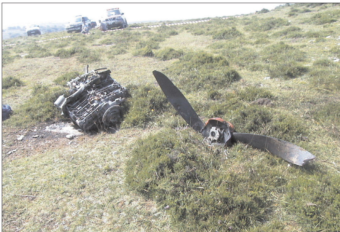
Figure C-3. Detached engine and propeller
