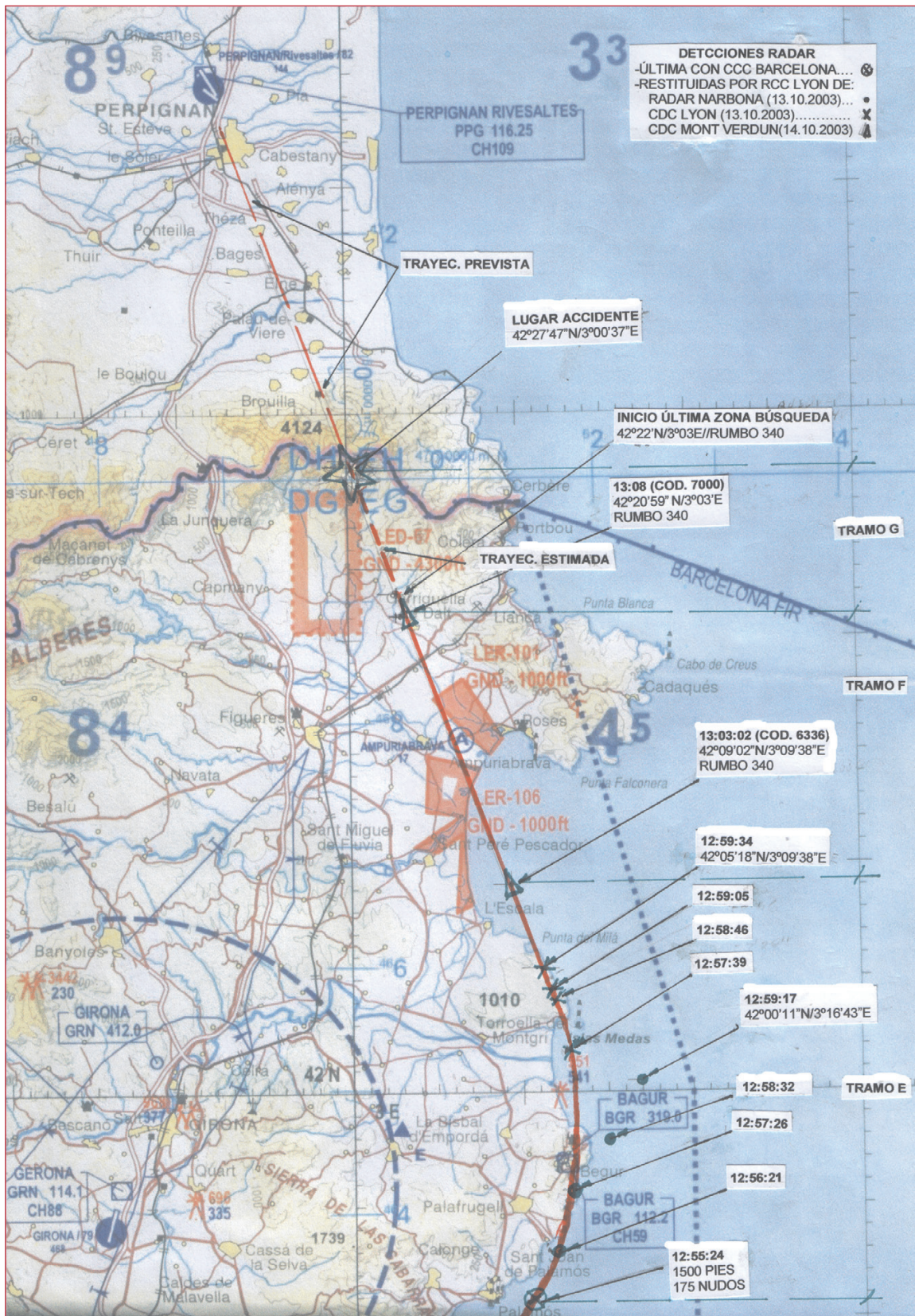
Figure B-2. Path amplified with rescue radar detections
