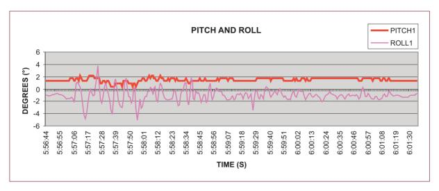
Figure 1.11.6. Pitch and lateral aircraft roll
