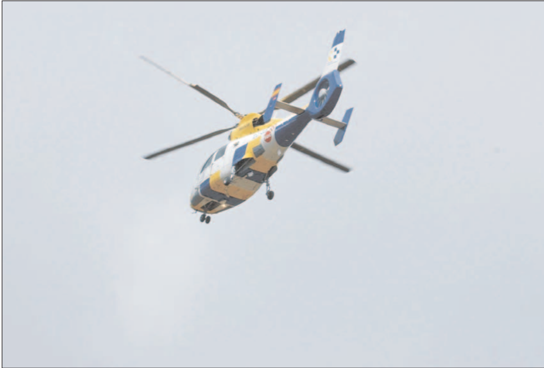
Figure 1.1.3. The helicopter flying shortly after the impact with the wires. Most of the chord of a blade is missing approximately in half of the span (photo «La provincia»)
