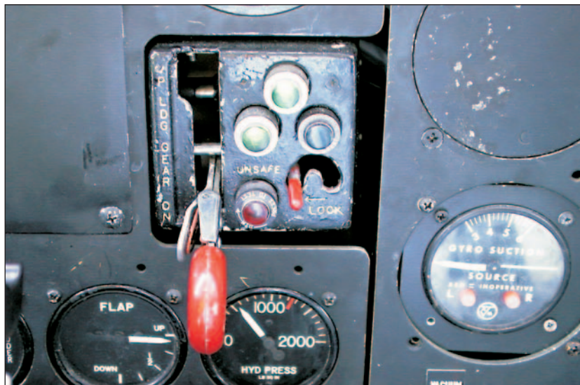
Figure 7. Landing gear lever and gear position indication lights
