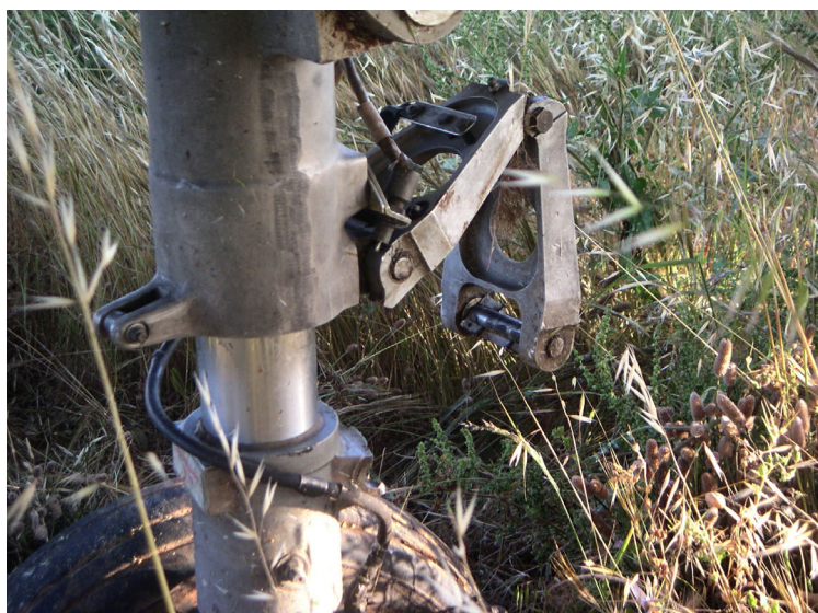
Figure 3. RH main leg. Breakage of the torsion link
