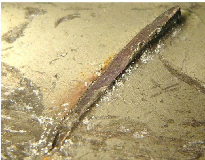
**Figure 9.** Fatigue failure of the vane
