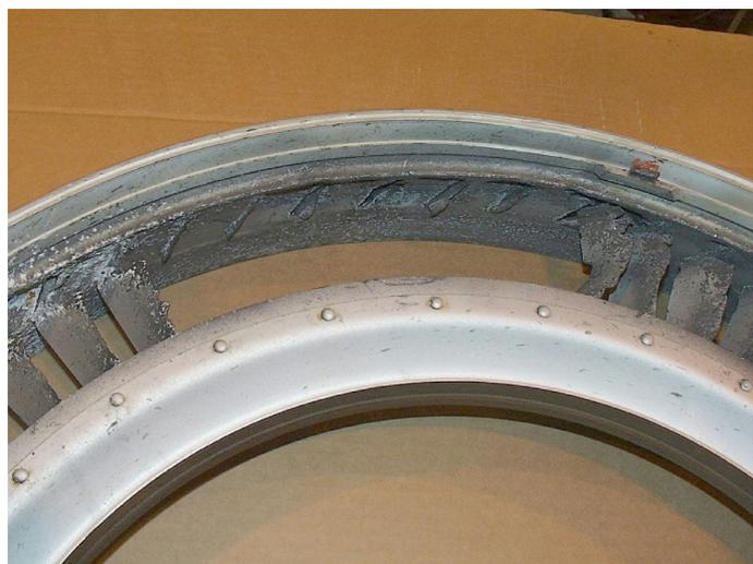
Figure 10. HPC 8th stage stator
