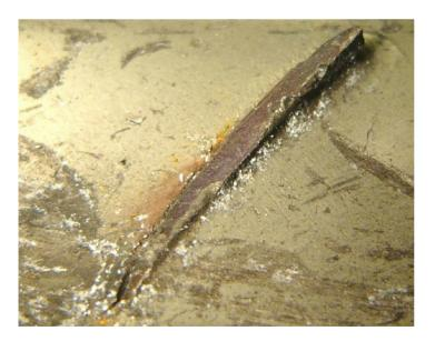
Figure 9. Fatigue failure of the vane
