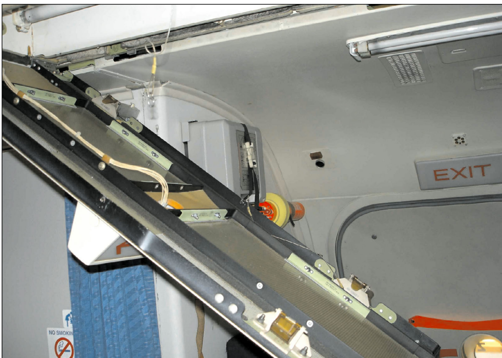
Figure 1.15.1.3. Ceiling panel in the rear cabin attendant compartment. During the inspection after the accident it was found closed, but witnesses stated that it opened after the aircraft came to a stop, therefore obstructing the path towards emergency exits L2 and R2. The lanyard released. The hook is at the end of the lanyard assembly
