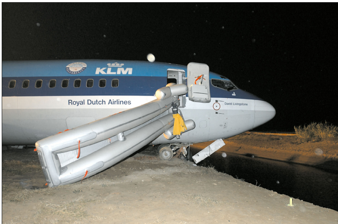
Figure 1.15.2. Escape slide of door 1R was twisted
