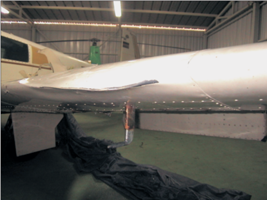
Photography 2. Damages to the left wing aircraft D-EIGB. Detail of the leading edge
