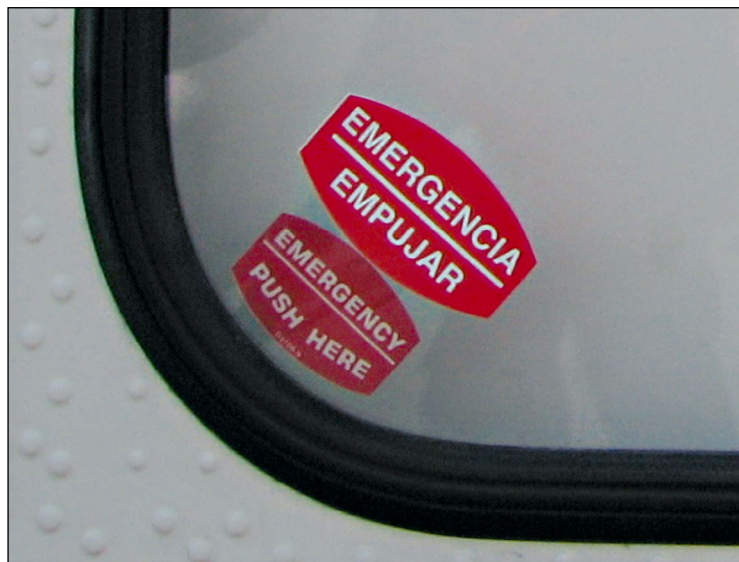
Figure 3. Stickers located on the lower corners of the emergency windows
