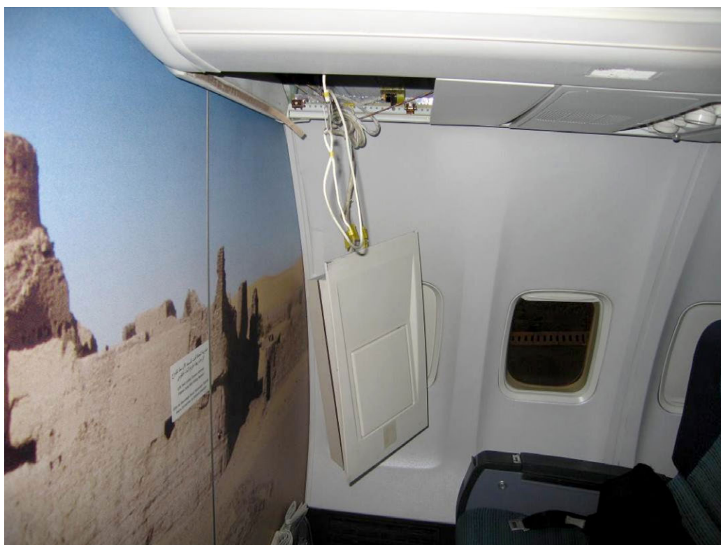
Photograph 6. Passengers cabin. Overhead panel detached
