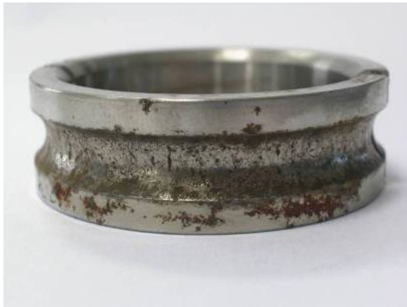
Figure 11. Example of the corrosion found on the inner race of the freewheel
