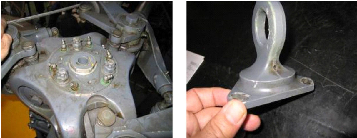
Figure 4. View of the top part of the mast and of the drilled component used on this type of helicopter
