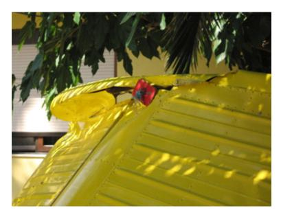
Figure 2. Pin installed in the left elevator
