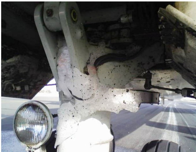
Figure 1. Picture showing ice in front gear wheel well
