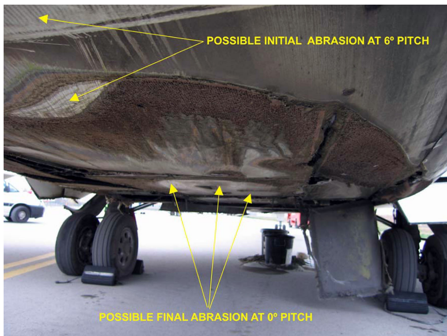
Figure 2. Abrasion marks, scrapes and distortions, on the aircraft belly
