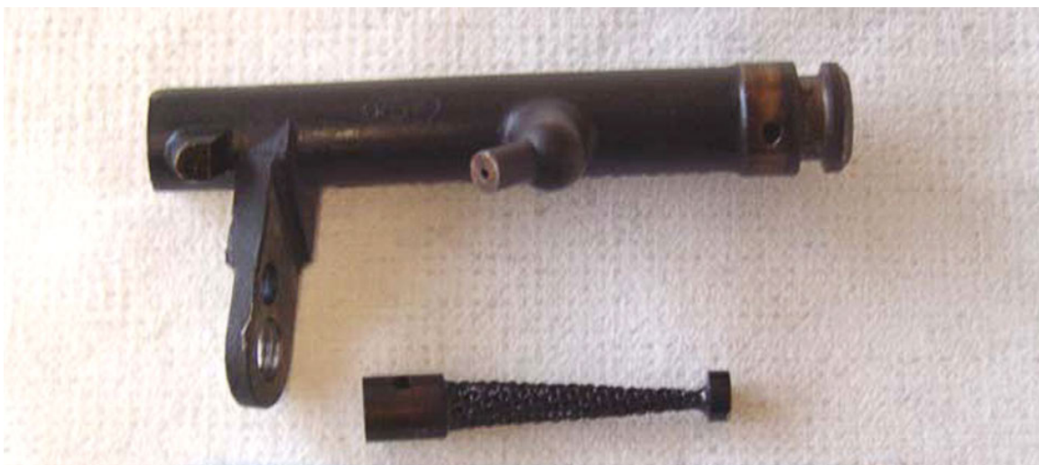
Figure 5. No. 2 bearing oil nozzle and oil nozzlestrainer
