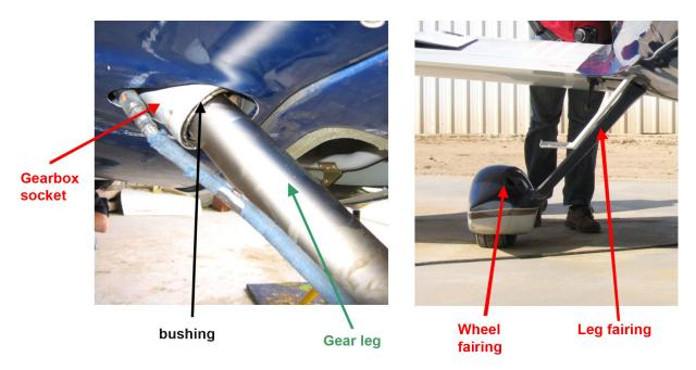
Figure 3. Close-up of gear structure
