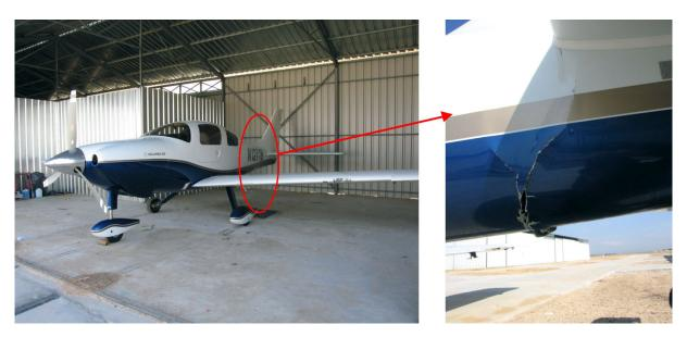
Figure 1. Close-up of the damage evident in the right wheel fairing and in the tail
