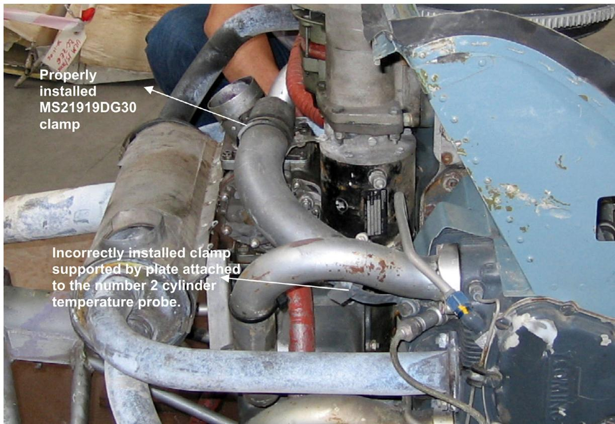
Figure 3. Alternative air tube installation
