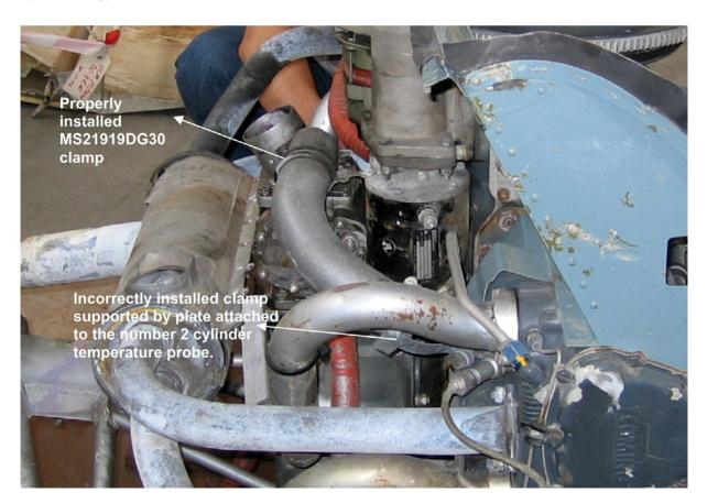
Figure 3. Alternative air tube installation
