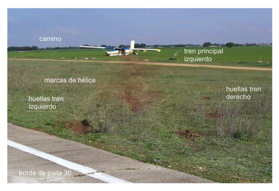
Figure 2. Marks and final aircraft resting place
