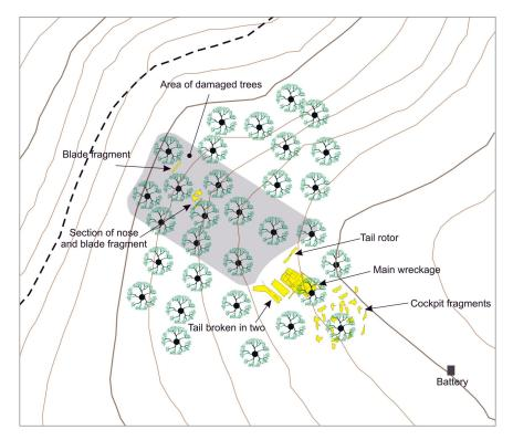
Figure 4. Diagram of debris field
