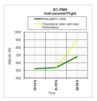
**Figure 6.** Graph of helicopter's climb during final moments o flight and theoretical climb applying the aircraft's maximum performance
