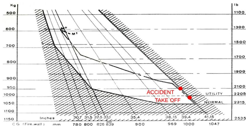
Figure 2. Position of CG during takeoff and accident
