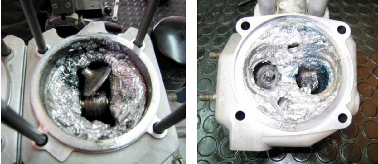
Figure 3. Condition of piston and no. 2 cylinder head
