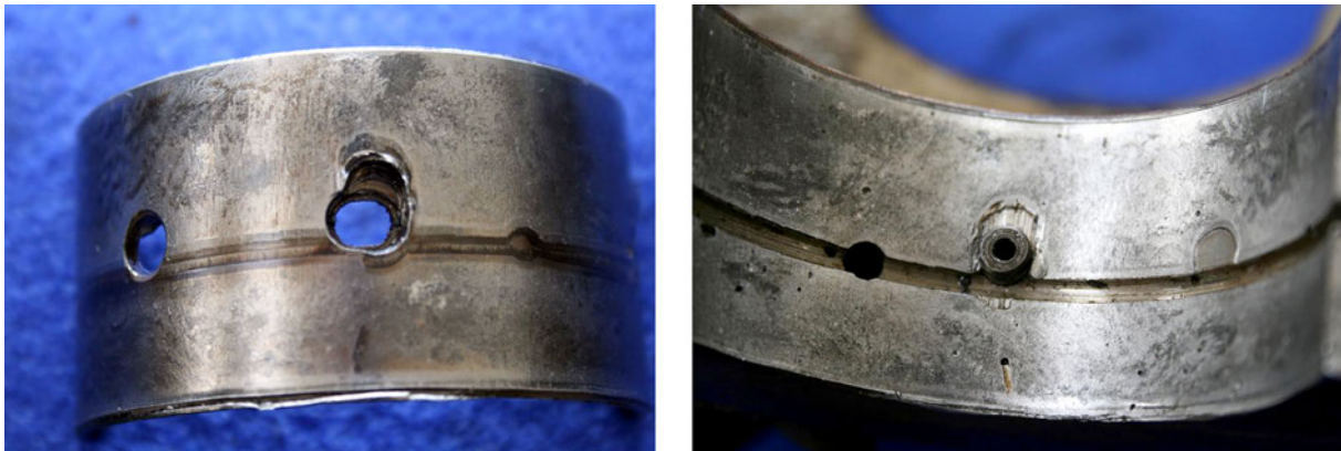
Figures 4 & 5. Deformations in the central half bearing and half casing
