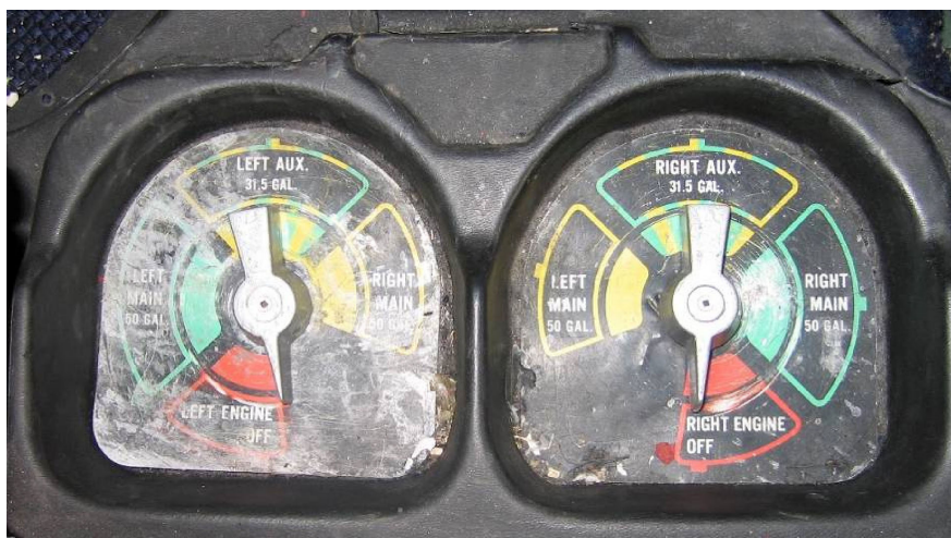
Figure 3. Fuel selector handles in the cockpit of an aircraft similar to that involved in this accident
