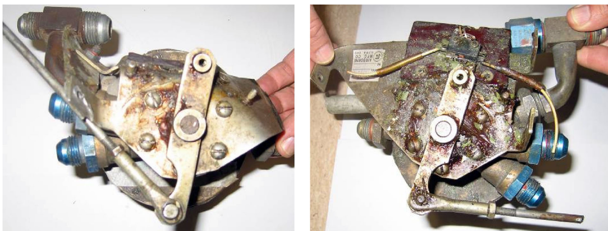
Figure 4. Fuel selectors inside the wings of the accident aircraft
