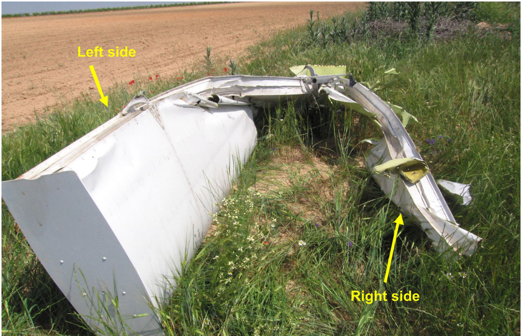
Figure 11. Photograph of the horizontal stabilizer
