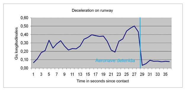
Figure 4. Deceleration during landing
