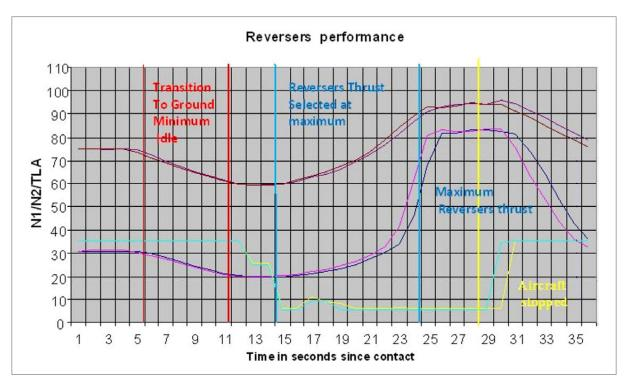
Figure 5. Engines performance during landing – reversers thrust
