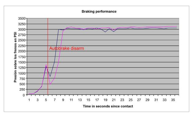
Figure 3. Braking performance during landing run
