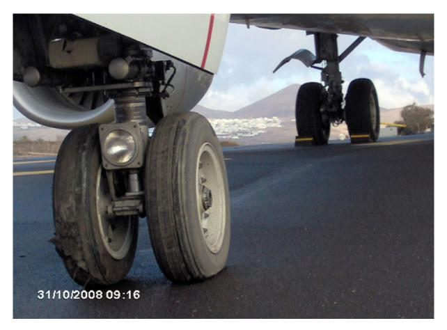
Figure 2. Damage to the nosewheel landing gear
