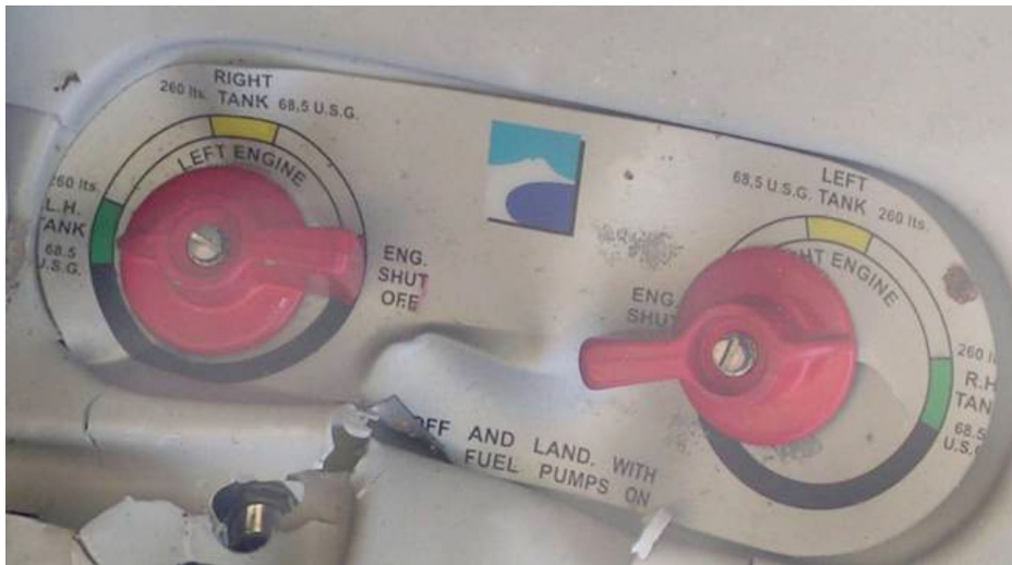
Figure 11. Fuel selector knobs
