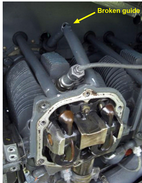
Figure 1. Photograph of broken guide
