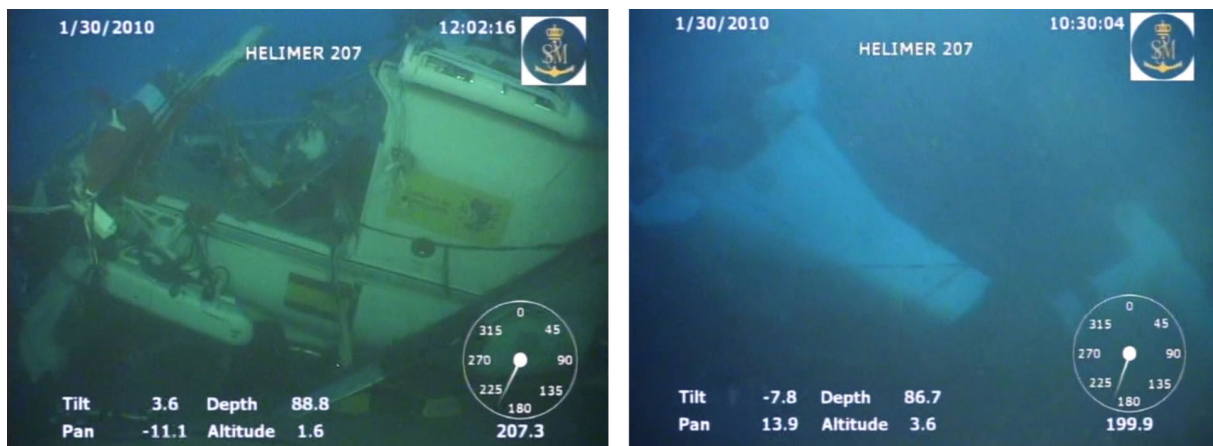
Figure 4. Condition of helicopter after impact. Images taken prior to recovery
