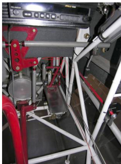
Figure 5. Areas near the pedals where the feet can become entangled
