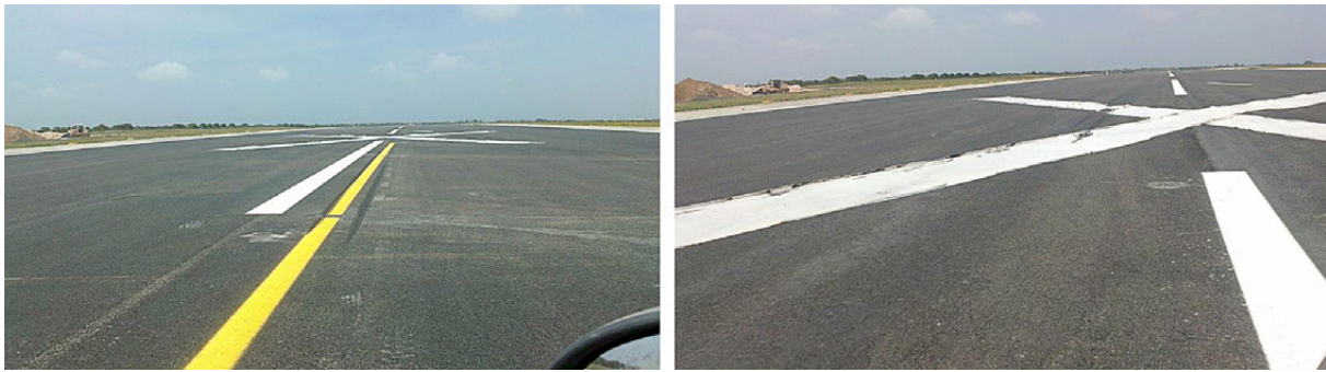
Figure 2. Landing marks, first from right gear and then from left, near the fourth runway-closed marking
