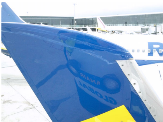
Figure 1. Damage to the B737 winglet
