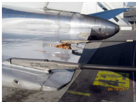
Figure 2. Damage to the B767 stabilizer
