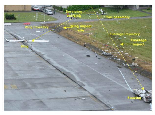
Figure 7. Photograph of wreckage taken from the runway
