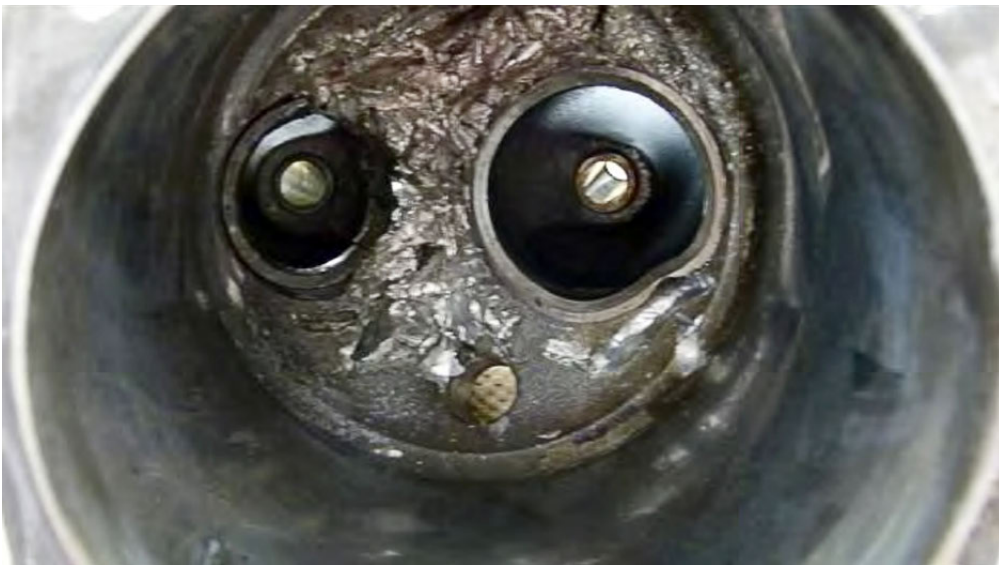
Figure 6. Interior of the no. 3 cylinder
