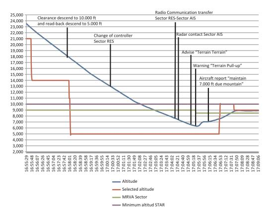
Figure 3. Flight profile of the aircraft during the incident
