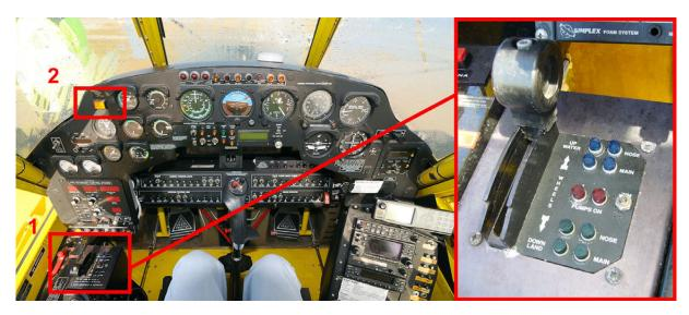
Figure 2. Location of visual gear indications in the cockpit of the AT802A
