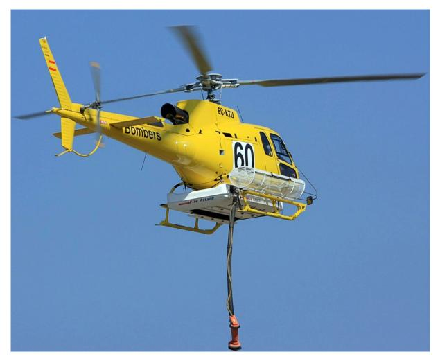
Figure 1. Helicopter with the Simplex 310 firefighting system attached
