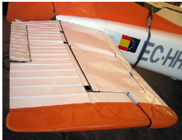
Figure 1. Damage to right stabilizer
