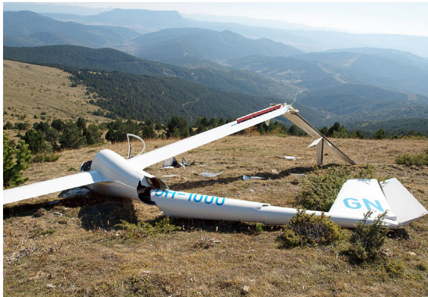
Figure 4. Detached tail assembly
