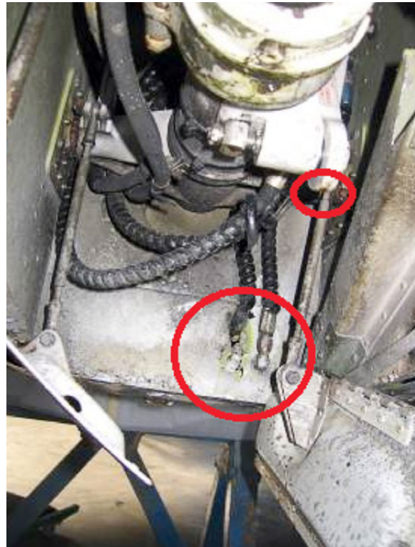
Figure 7. Impact on the rear bulkhead and part of the leg responsible for the impact
