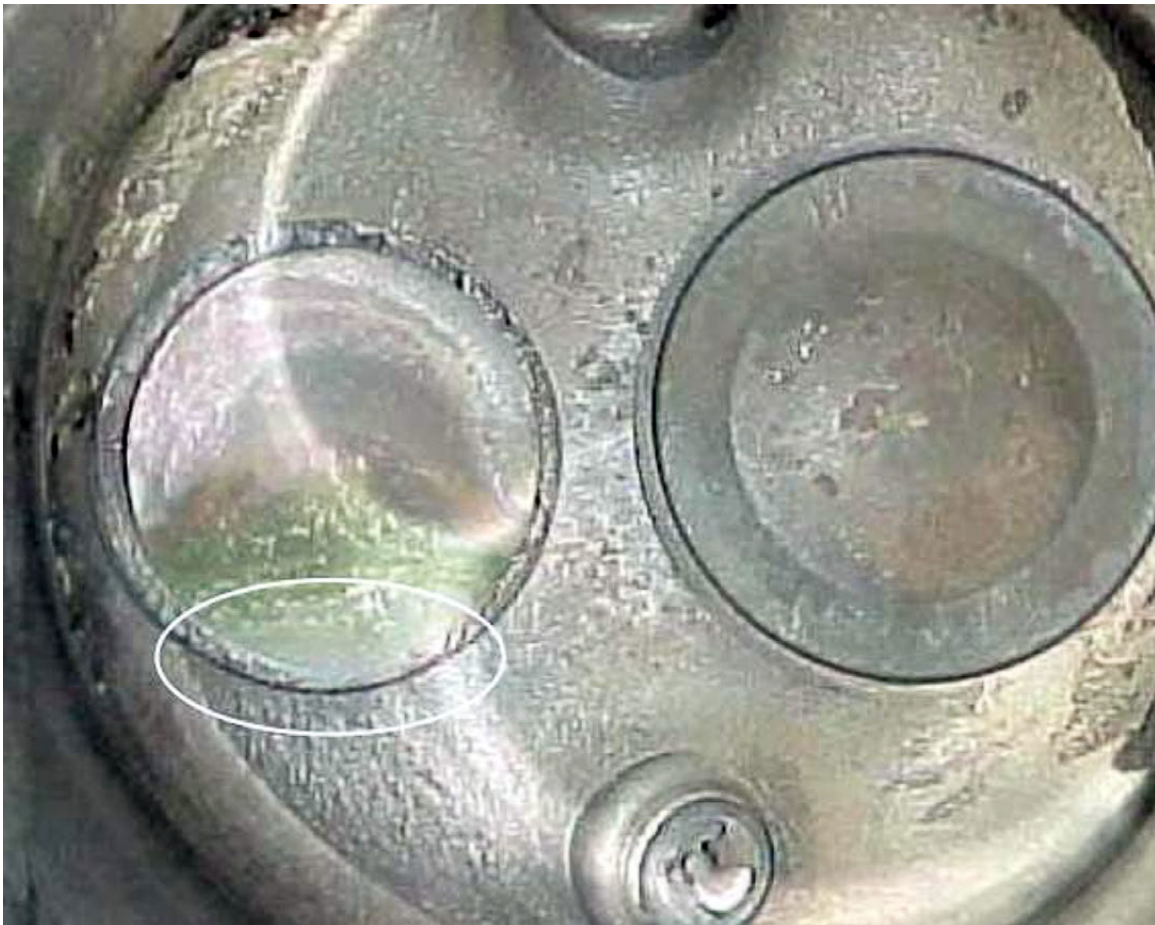
Figure 7. Taken from SB03-03 by TCM. Shows a burned exhaust valve with signs of leakage and damage
