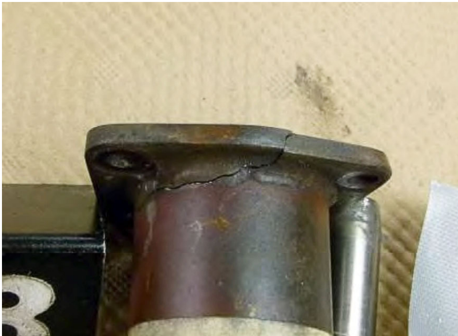
Figure 4. Cracks and signs of overheating in the no. 3 exhaust port.
